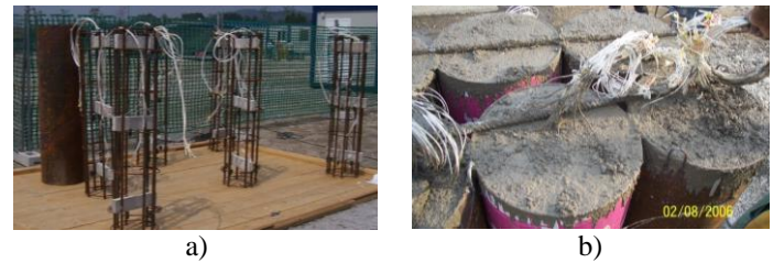
Figure 1. Bergamo Hospital site: a) steel cages with Chromel-Alumel thermocouples; b) Specimens Cast
