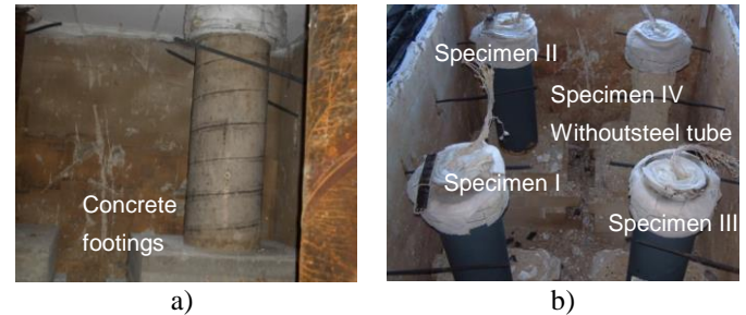
Figure 3. CSI Fire Tests: a) Specimens in the furnace before heating standard process; b) Specimens in the furnace after heating standard process
